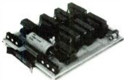
MODEL 212 1 x 6 DA, 6 individual balanced transformer outputs $150.00
